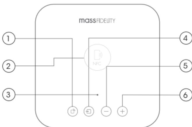
1. **MULTI-ROOM key:** transmit audio from this unit to additional Core speakers for multi-room audio
